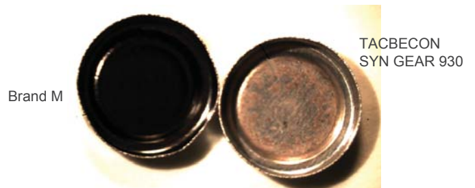
Image 6. Comparison of Deposits Formation after Complete Decomposition at High Temperatures.
